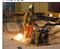
Anatomy of structural failure: The UL tests included two 300-lb mannequins to simulate a pair of firefighters in protective gear. In this photo, the basement fire below is causing the supporting joists to weaken; note the bowing of the floor.
