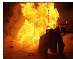
A mannequin crashes through the floor as the supporting joists fail.
