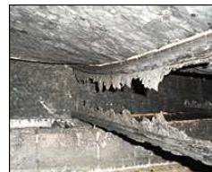
The view from below after a test, with the center of an engineered I-joist almost completely burned away by fire. (Photos: Underwriters Laboratories)
